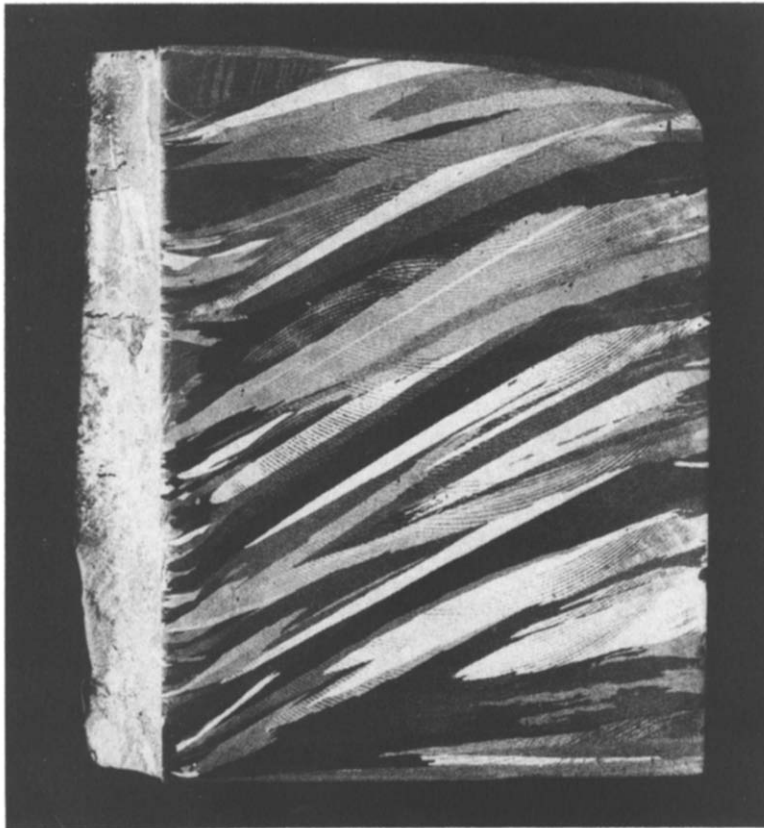
FIG. 12. Macrostructures of commercially pure tin (vertical slices) solidified in natural convection, (a) \Delta T = 100^\circ\text{C} , in the presence of a forced Couette flow, (b) \Delta T = 100^\circ\text{C} , \omega_c = 13.23 \text{ rad s}^{-1} , and in the presence of crossed electric and magnetic fields, (c) \Delta T = 100^\circ\text{C} , M = 80 , I_0 = 250 \text{ A} .
